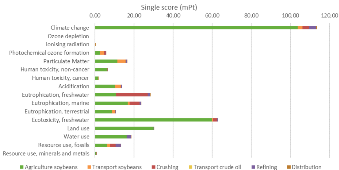
Figure 97: Weighted environmental profile of 1 tonne acid oil, deodistillates or fatty acid distillates from soybeans
