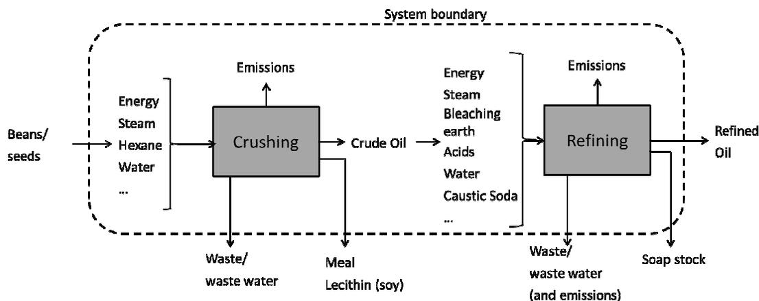
**Figure 1: System Boundary : Crushing and Refining**
