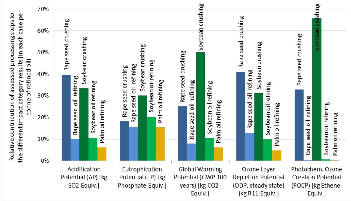
**Figure 2: Relative LCIA results for the five environmental impact categories per tonne of refined oil**
